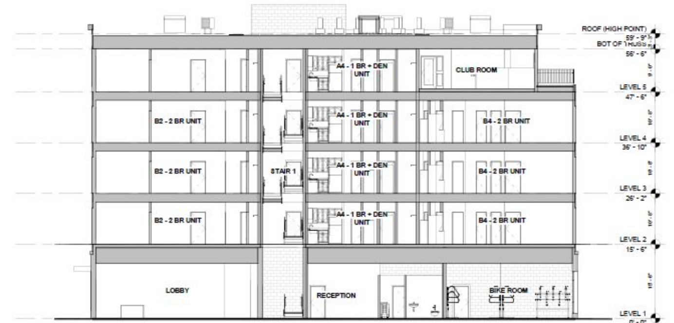
1 BUILDING SECTION 1 Scale: 1/8" = 1'-0"
