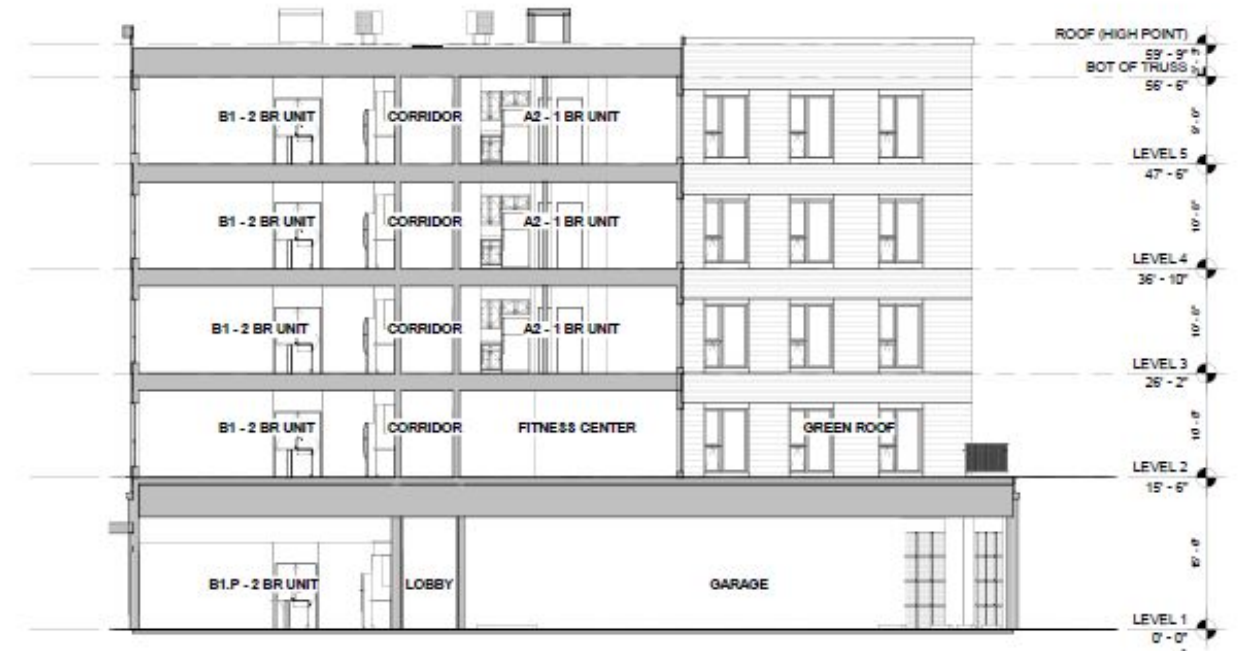
2 BUILDING SECTION 2 Scale: 1/8" = 1'-0"
